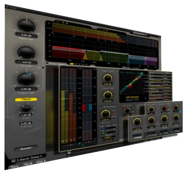
At first, the wideband signal is split into frequency bands by a slope adjustable cross-over.
