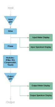
Figure 1.1: EVO Channel architecture
