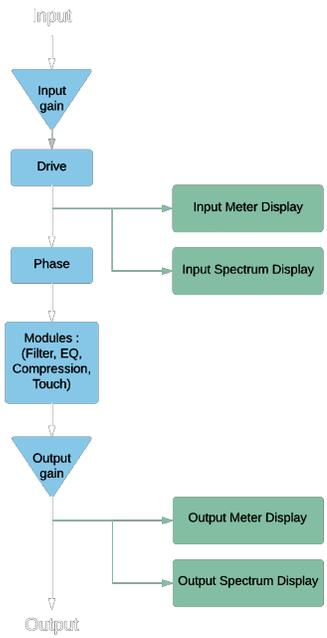
Figure 1.1: EVO Channel architecture
