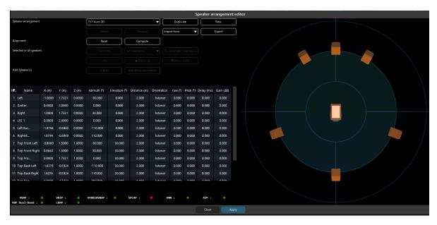
Figure 18.1: The speaker arrangement editor window showing a predefined 13.1 Auro 3D speaker arrangement.
