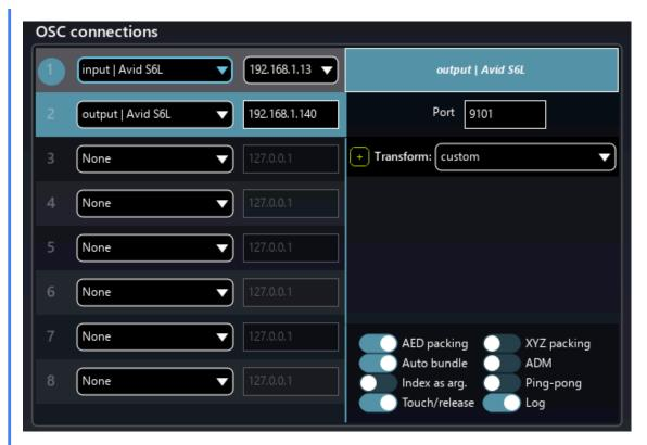
Figure 49.3: SPAT OSC Connections Matrix
